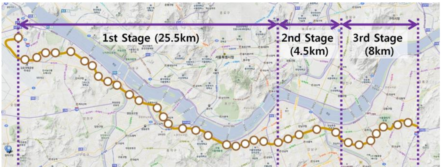
<Figure 1> Construction Sections of Subway Line 9
