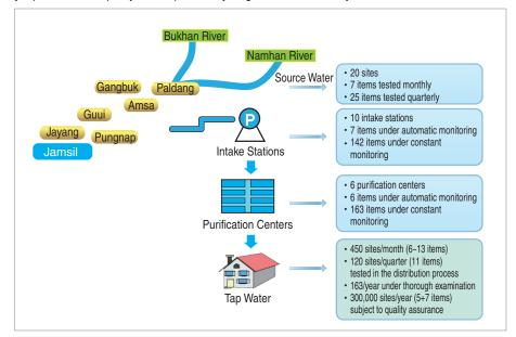
Setting up an automatic water quality monitoring system for both source water and raw water at intake points
