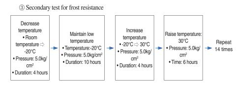
% Conduct a flow test after repeating the process above for 7 out of 14 times.
