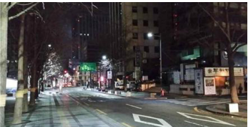
20% brightness when there is no vehicle on the road
